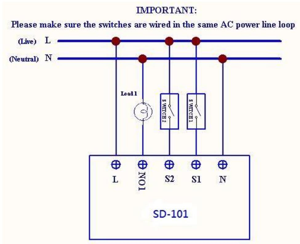
Fig 1. Assembling & Wiring
